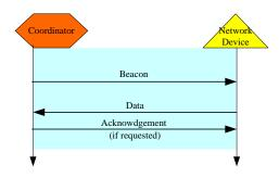
Fig. 6. Data transfer to coordinator (reproduced from [15]).
