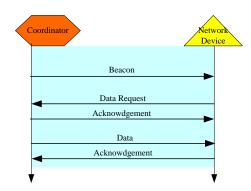
Fig. 7. Data transfer from coordinator (reproduced from [15]).
