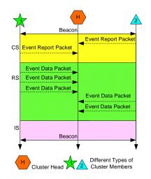
Fig. 8. The packets sequence diagram in App-MAC.
