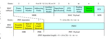
Fig. 3. The beacon frame in IEEE 802.15.4 (reproduced from [15]).
