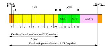
Fig. 2. The superframe in IEEE 802.15.4 (reproduced from [15]).
