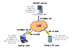
Figure 5. A simplified UbiCAS system deployment and configuration.
