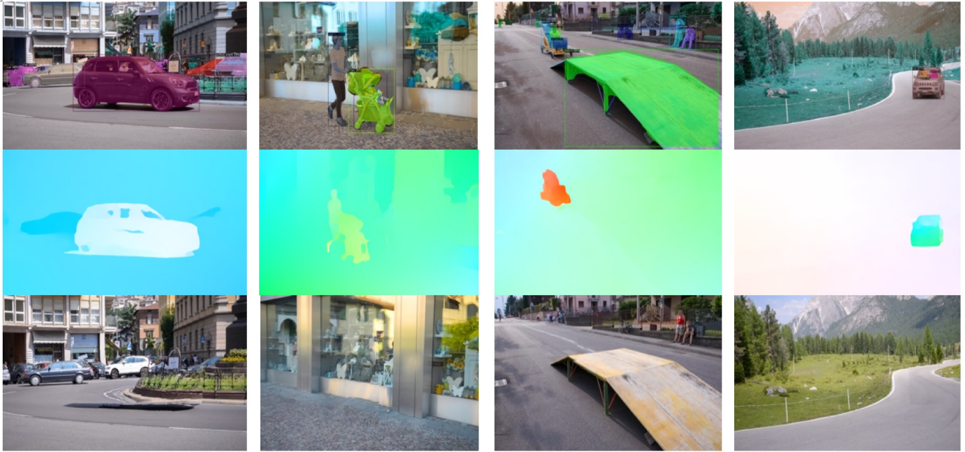
Fig. 1: Different steps of object masking and removal, the first row demonstrate the object mask and label, the second row is visualized optical flow, and third row is the final result for inpainting.
