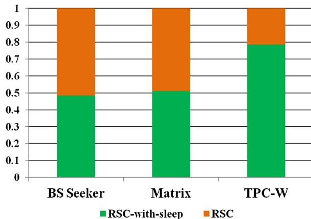
**Fig. 6.** Normalized average energy savings with sleep state enabled.
