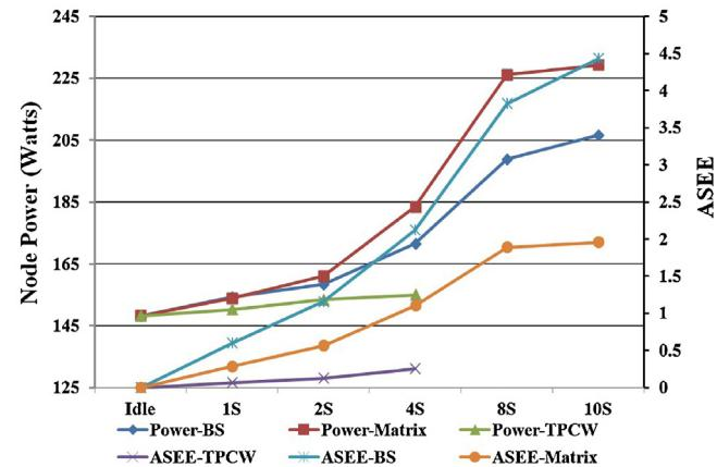
Fig. 2. The power and ASEE of running 1, 2, 4, 8, and 10 Small VMs on Node-2.
