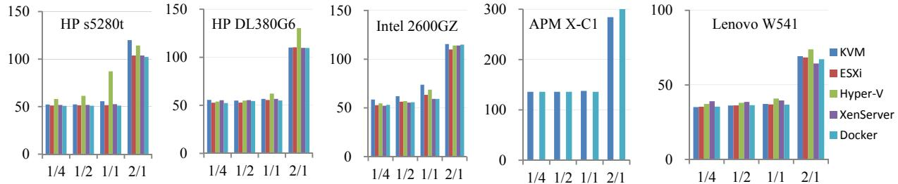
**Fig.2** Completion time of varying computing workloads (x axis: workload level, y axis: completion time (10^3 seconds))
