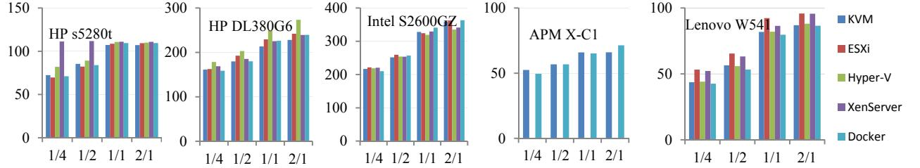
(a) Power consumption (x axis: workload level, y axis: power (watts))
