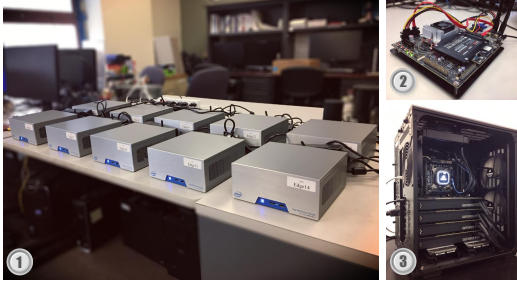
Fig. 2. Three categories of hardware. Subfigure 1-3 shows the Intel Fog Reference Design (FRD), Jetson TX2, and NVIDIA GPU Workstation, respectively.
