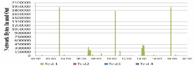
Fig. 7: Network Bytes In and Out of iPhone using Wi-Fi
