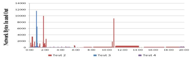
Fig. 10: Network Bytes in and Out of iPhone using 3G excluding Test 1
