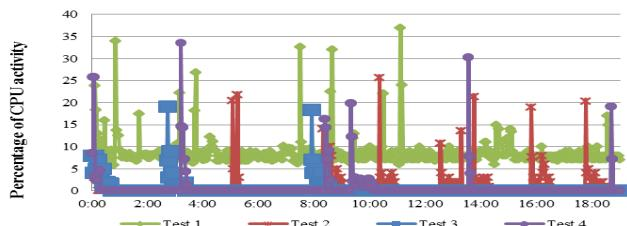
Fig. 5: Percentage of CPU activity of iPhone using Wi-Fi
