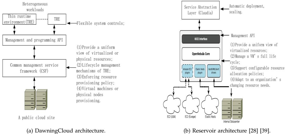
Fig. 2: The architectural differences between DawningCloud and Reservoir.
